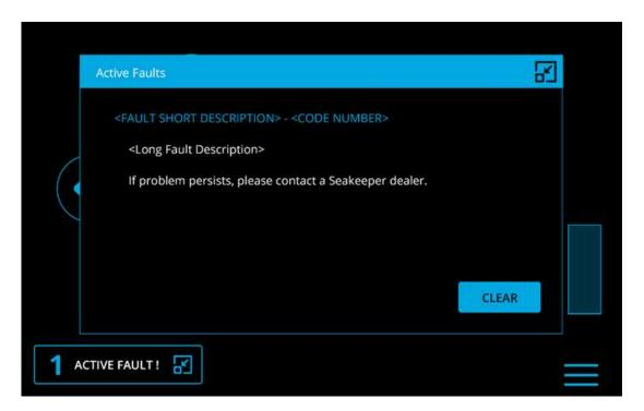
The Fault History page on the Seakeeper Application shows the recent faults and warnings. Faults trigger a pop-up message to be displayed on the Seakeeper Ride application and cause the Keypad to be non-responsive. Warnings will be listed in the fault history but do not affect operation. The history of faults and warnings are in chronological order starting with the most recent. To show the
